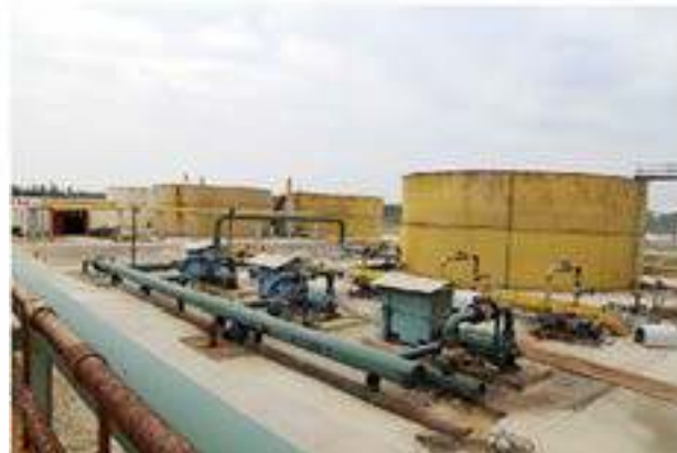
中盐集团采卤泵、输卤泵应用现场 (型号: DF280-65×10 数量: 6台套) China National Salt Industry Company brine extraction pump working site (Model : DF280-65X10, 6 sets)
